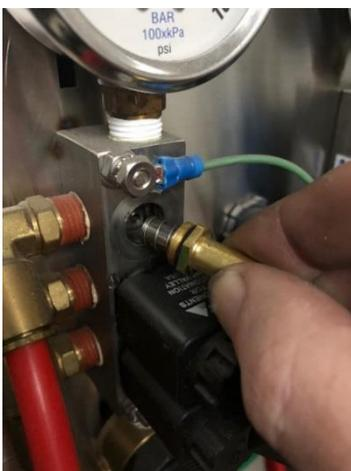
If you can't hear a click it could be a faulty coil or actuator stuck in the stem, the majority of the time it's the stem that is faulty.
